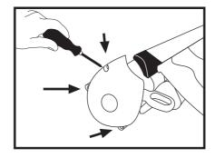
2. Remove the three screws located at side awning (lid). NOTE: usually hidden under a sticker.
