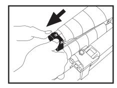
4. Remove the end cap located by the end of the valance. You will see two more screws, remove along with plug/bung.
