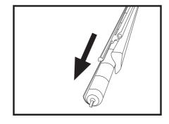
7. Slide the fabric roller out of the frame.
