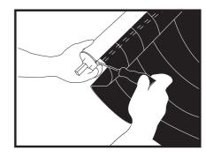
12. Tighten up the screw plug/bung.
