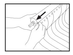
**9.** One more screw/bung to remove, located by the end of the fabric/roller. This keeps the fabric in place.
